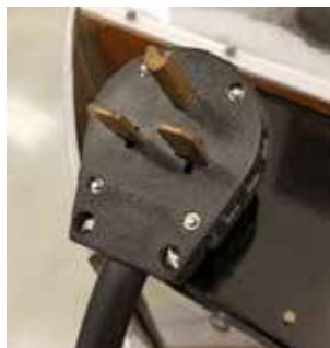
Receptacle / Plug Config. & NEMO no. 6-30
