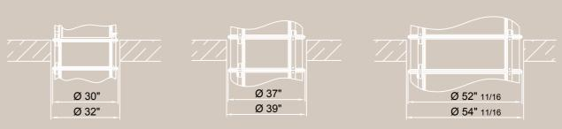
Minimum diameters for finished holes in through-floor installations.
